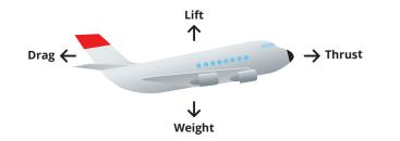
Four forces; thrust, lift, drag and weight are needed to make a plane fly.
